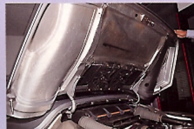
Engine cover is a complex Kevlar moulding – and terrifyingly expensive!
