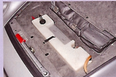
The battery is situated below the large washer reservoir. Note cut-out switch
