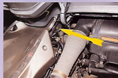
Cylinder-head coolant is topped up when necessary through this filler cap
