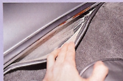
Chassis number is stamped on right-hand inner wing, behind the carpet
