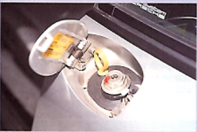
A special tool is needed to top up the transmission fluid (above)
