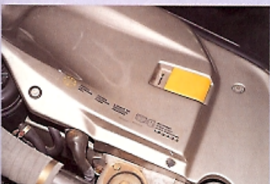
This latch (above), to the right of the engine, releases the engine-oil filler flap
