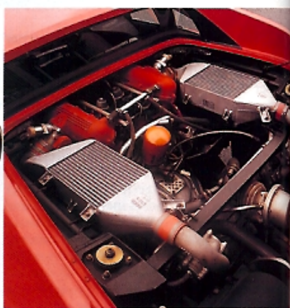
Above (l-r): clinical 959 engine bay conceals clever internals; perfect aerodynamics give zero-lift; massive intercoolers dominate 288 unit. Far left: '77 PF Millechiodi concept
