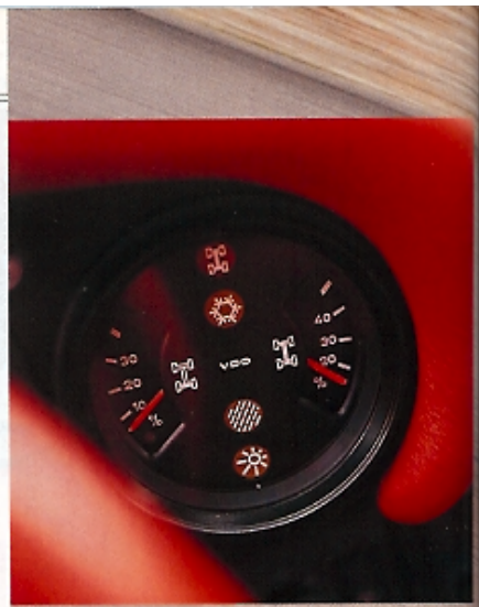
Clockwise, from top left: tyres can run flat on hollow Porsche alloys; showy Speedline split rims for Ferrari; 959 dash shows percentage of drive to front and rear; its graceful if useless mirrors; clumsy but effective on 288; huge complexity of 959
