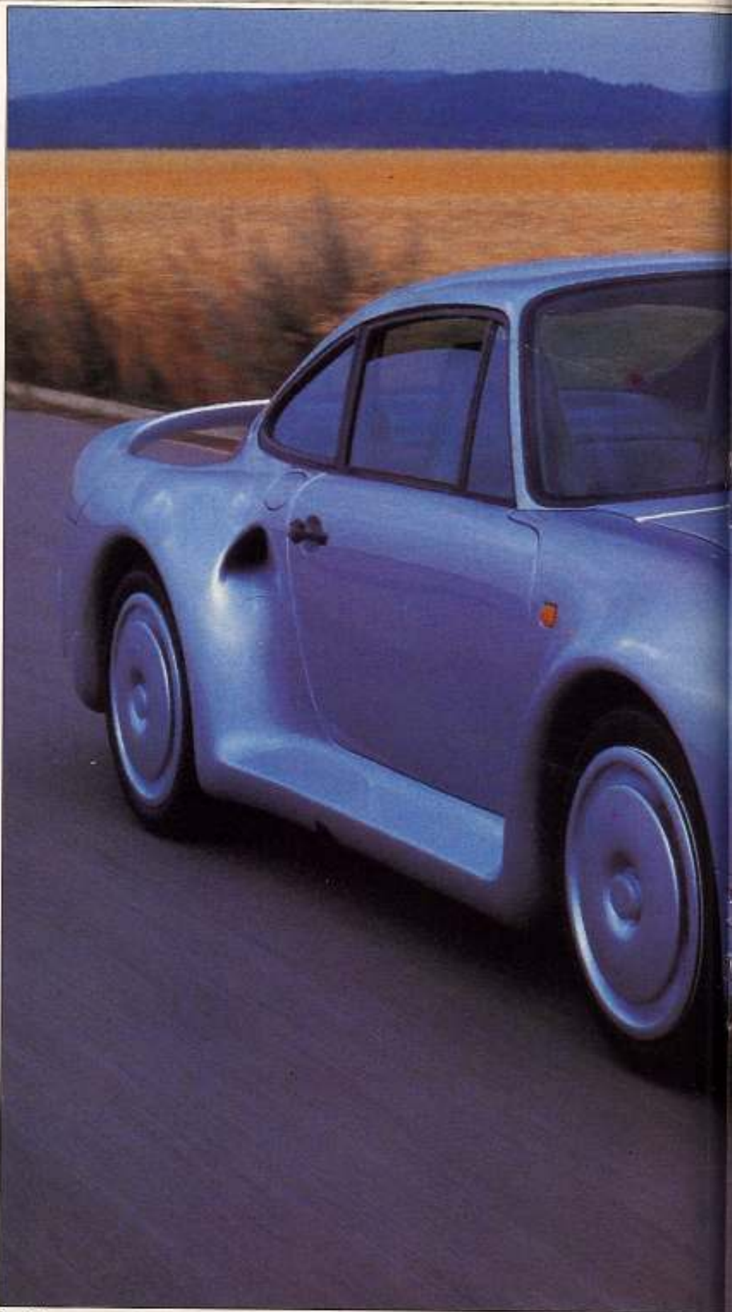
Special cast magnesium wheels include tyre pressure sensors, with dashboard read-out
